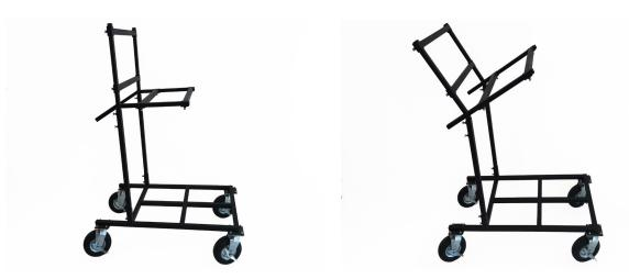
The Double Stack Speaker Rack will hold any size bass speaker cabinet on the bottom and any size mid range horn speaker on top. The top speaker tray can be set in a flat or 30° angle. The 8 inch locking, swivel Flat Free Tires allow it to turn on a dime.
